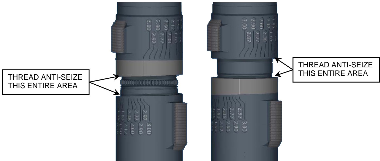
Figure 3: A) Spacer ring ready for engagement at 3 degrees. B) Spacer ring engaged at 3 degrees
