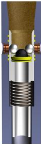
De-Activation Balls Dropped PRESSURE UP
