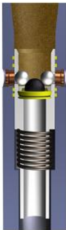
De-Activation Balls Dropped PRESSURE UP
