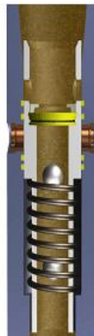
Balls Sheared Thru Seat Tool Reset
