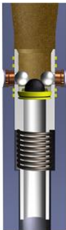
De-Activation Balls Dropped PRESSURE UP
